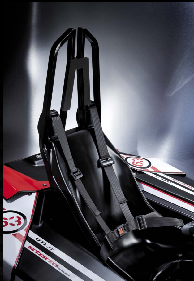
Seat belts and roll-bar according to DIN standards.
